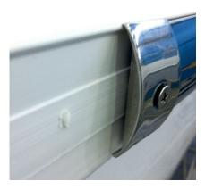
The drill spindle must not touch the countersink of the screw: we recommend inserting a plastic or aluminum stop buffer on the drill bit; this simple operation will prevent the iron material of the spindle from damaging the steel. It is advisable to apply silicone to the hole making screwing smoother and sealing the hole itself.
