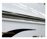
Then cut the side strips to the correct size and complete the installation using the supplied joint covers.
