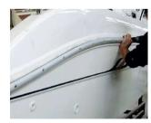
Small side bends can be performed directly on the boat.
