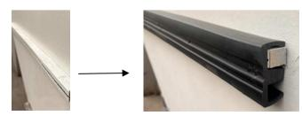
The base can be mounted on boats with a sandwich junction by positioning the recess either above or below according to need. The recess has a depth of 22 mm and a height of 18 mm.
